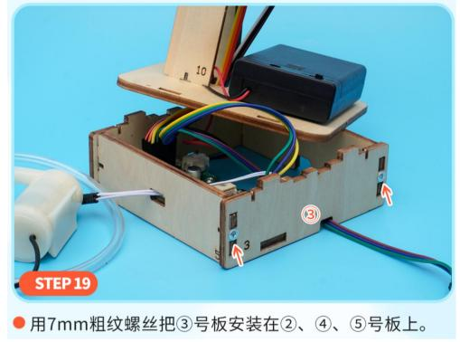
STEP 19. Install board 3 on boards 2 , 4 , and 5 with 7mm coarse thread screws.
