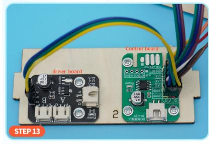
Insert one end of the 10cm Dupont cable into the O|PWM interface on the control board, and insert the other end into the basic driver board.
