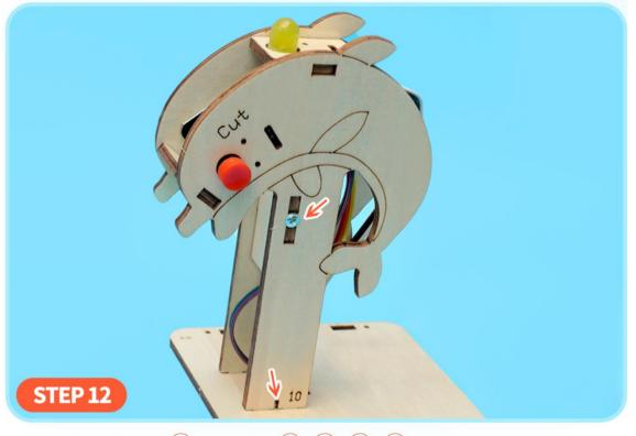
First, install board 10 on boards 1, 6, 7, 8,and then fix board 10 on boards 1, 8 with 7mm coarse thread screws.
