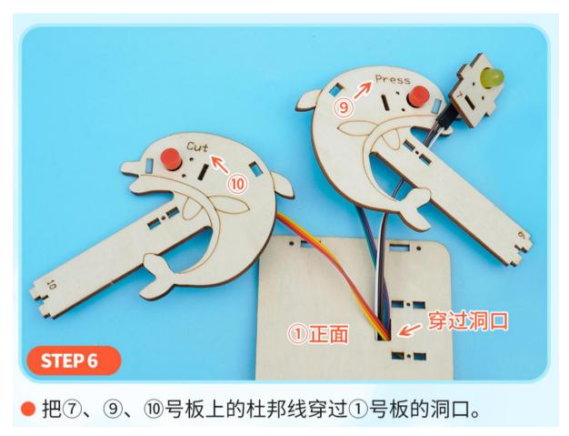
STEP 6. Pass the Dupont wires on boards (7, 9), and (10) through the opening of board (1) (Front-side).
